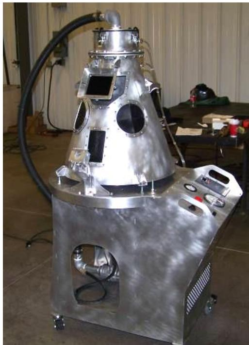
**Figure 1. NSRP Weld Fume Chamber**
