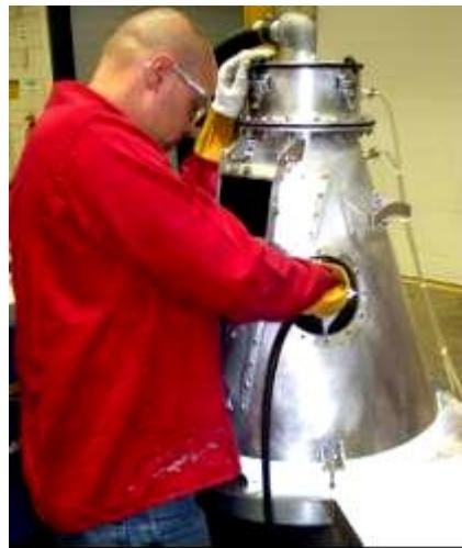
**Figure 8. Welding Inside Weld Fume Chamber**
