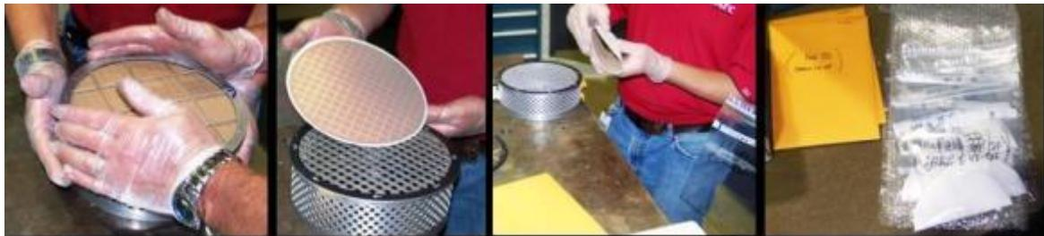
**Figure 12. Removing Fume Sample from Weld Fume Chamber**
