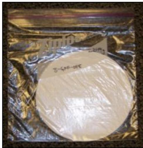
**Figure 4. Filter in Labeled Bag**
