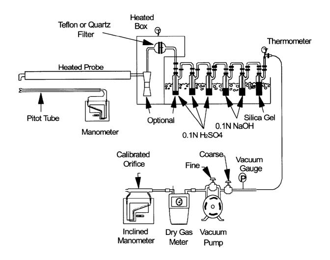
Figure 1. Sampling Train for Methods 0050 and 26A.
