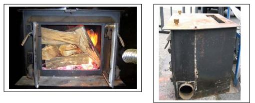
**Construction:** The unit is constructed primarily of heavy gauge steel. The firebox has a cement base. The firebox dimensions are: W 22 in x L 14.9 in x H 17.5 in (W 50.8 cm x L 37.8 cm x H 47.0 cm). The firebox in surrounded by an air circulation area. The feed doors are cast iron and have two  $\frac{1}{2}$  in (1.3 cm) flat braided fibreglass gaskets.
