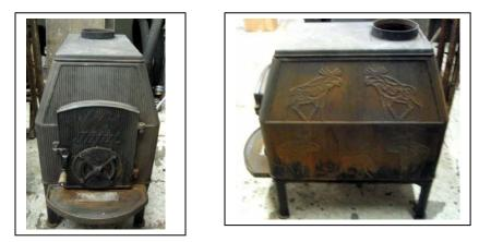
**Construction:** The unit is constructed primarily of cast iron. The unit has a separate cast iron firebox lining. The firebox dimensions are: W 11 in x L 25.5 in x H 15.25 in (W 27.9 cm x L 64.8 cm x H 38.7 cm). The feed door is cast iron with  $\frac{1}{4}$  in (0.625 cm) braided rope gasket.
