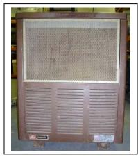
**Construction:** The unit is constructed primarily of mild gauge steel. The firebox is lined with firebrick. The firebox dimensions are: W 11 in x L 17.5 in x H 19.5 in (W 28 cm x L 45 cm x H 50 cm). There is an outer steel shell, with vents, enclosing the unit. The feed door and ash door have 7/8 in (2.2 cm) fibreglass rope gaskets.
