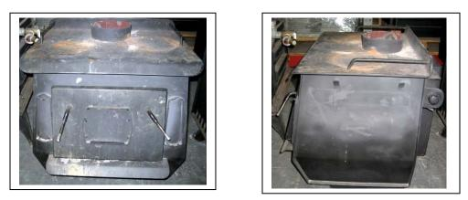
**Construction:** The unit is constructed primarily of mild steel. The firebox is lined with firebrick. The firebox dimensions are: W 16 in x L 13.5 in x H 15.75 in (W 40.6 cm x L 34.3 cm x H 40.0 cm). The feed door has 1.5 in (3.8 cm) braided fibreglass rope gasket.
