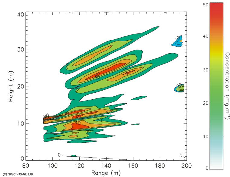
**Figure 5: Visual indication of methane leak at gas plant B.
