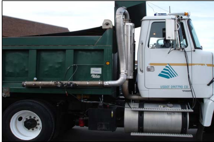
Figure 2. Calibrated flow pipe installed
