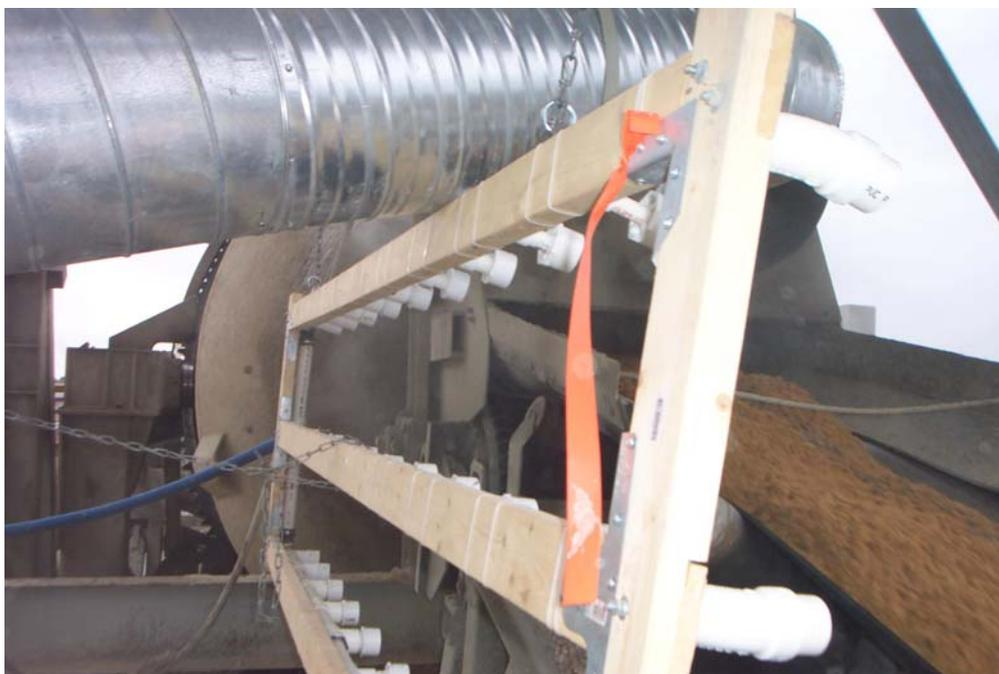
Figure 2. Sampling Array at the Inlet of a Central Mix Operation
