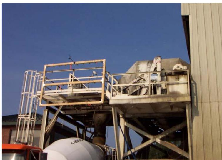
Figure 3. Sampling Array at the Outlet of a Central Mix Operation
