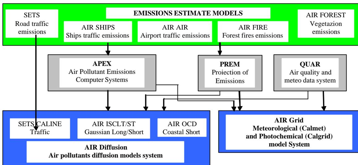
Figure 1: Structure of information system for air quality management planning
