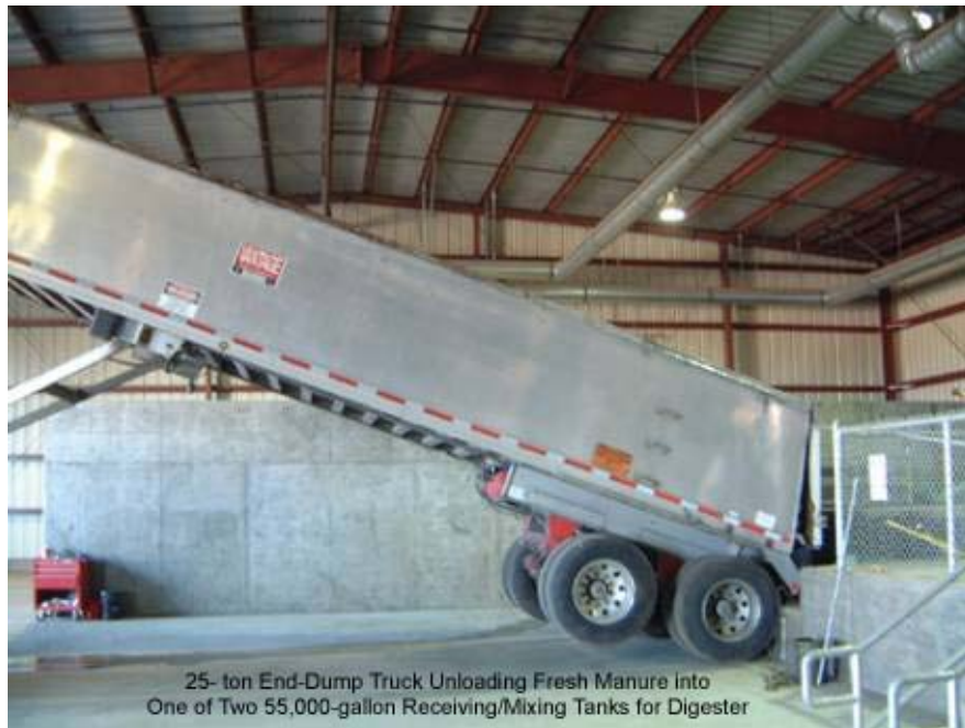
Figure 4. End dump unloading manure at RP-5.
