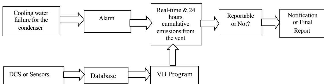
Figure 3. Flow Diagram For Upset Emissions Calculation
