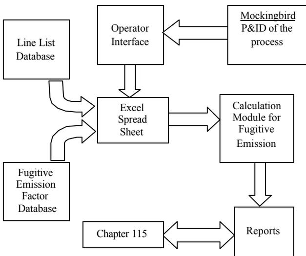
Figure 2. Flow-diagram for fugitive emissions calculation
