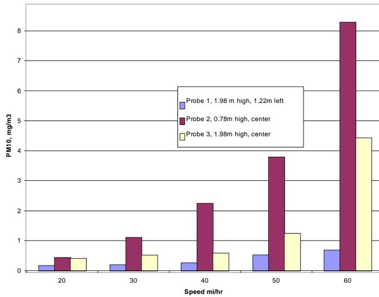
**Figure 7.** PM<sub>10</sub> concentrations while towing the test trailer at various speeds with two of the isokinetic sampling probes located 102 inches (2.59 m) above the ground.
