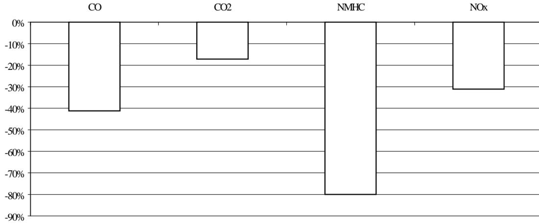
**Figure B.2. Heater/Boiler Conversion from Oil to LPG**
