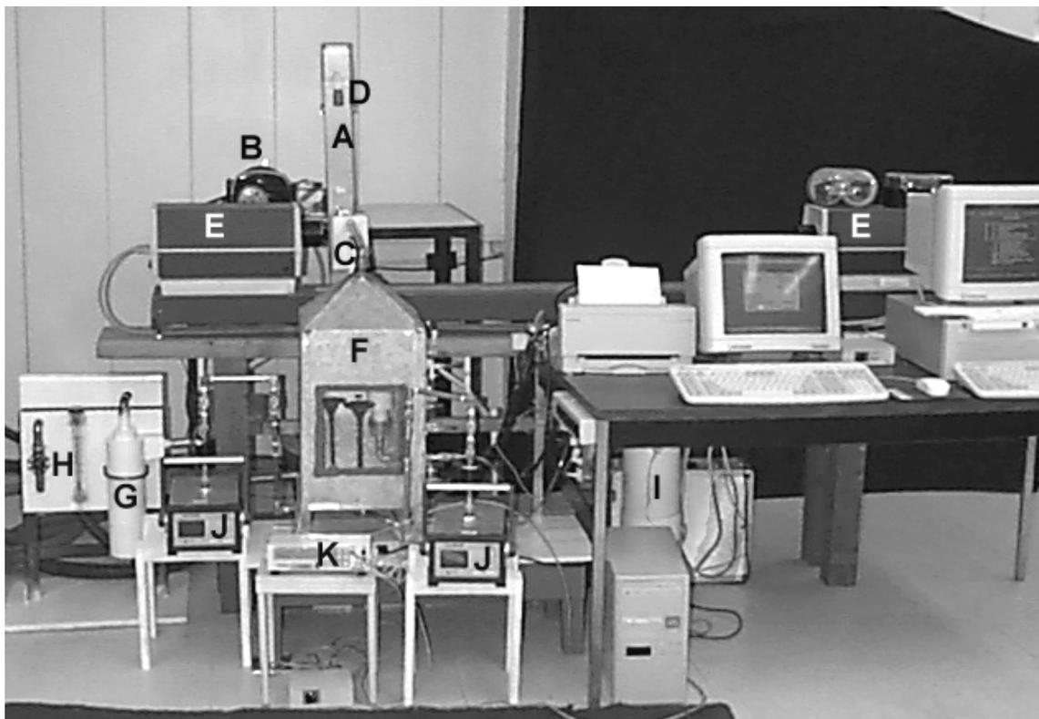
**Figure 1.** The Lubbock Dust Generation, Analysis and Sampling System.
