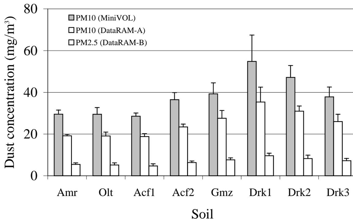
**Figure 2.** Aerosol PM<sub>10</sub> and PM<sub>2.5</sub> concentrations as measured by the MiniVol and DataRAMs dust monitors.
