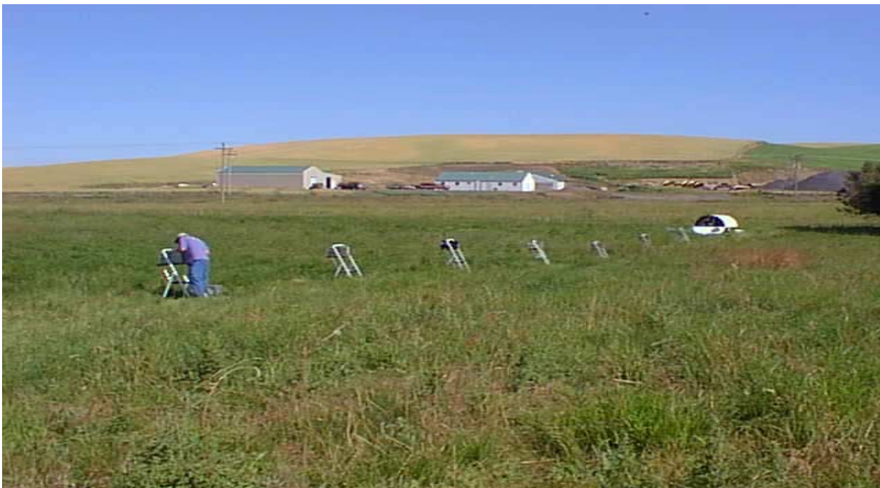
Figure 5. The line of \text{SF}_6 syringe samplers in operation along a 70m absorption path. Lagoon #2 is upwind to the left of the picture approximately 100m.
