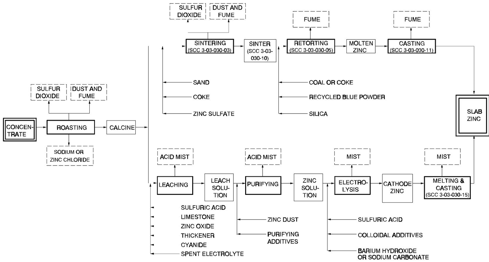
Figure 12.7-1. Generalized process flow for primary zinc smelting. (Source Classification Codes in parentheses.)
