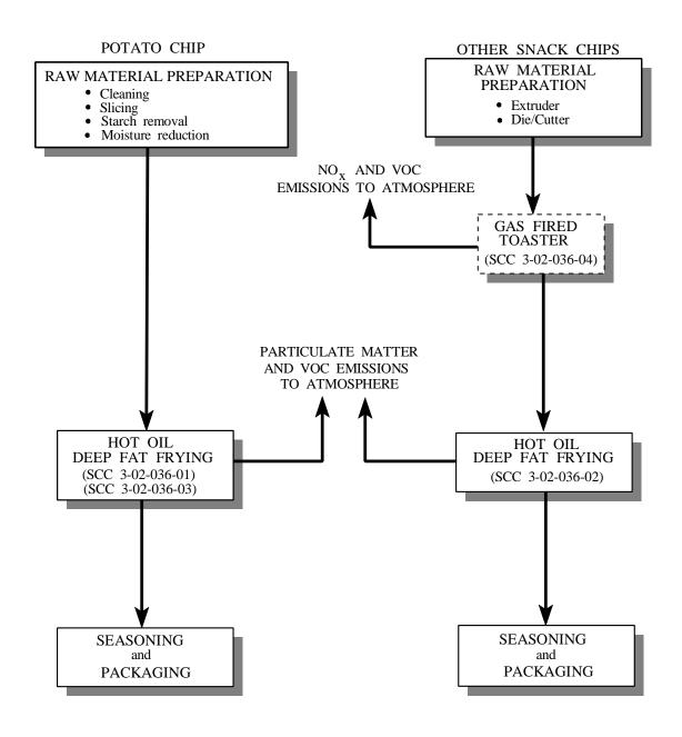
Figure 9.13.3-1. Generalized deep fat frying process for snack foods. (Source Classification Codes in parentheses.)
