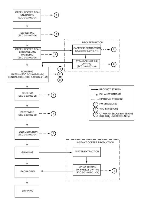
Figure 9.13.2-1. Typical coffee roasting operation. (Source Classification Codes in parentheses.)
