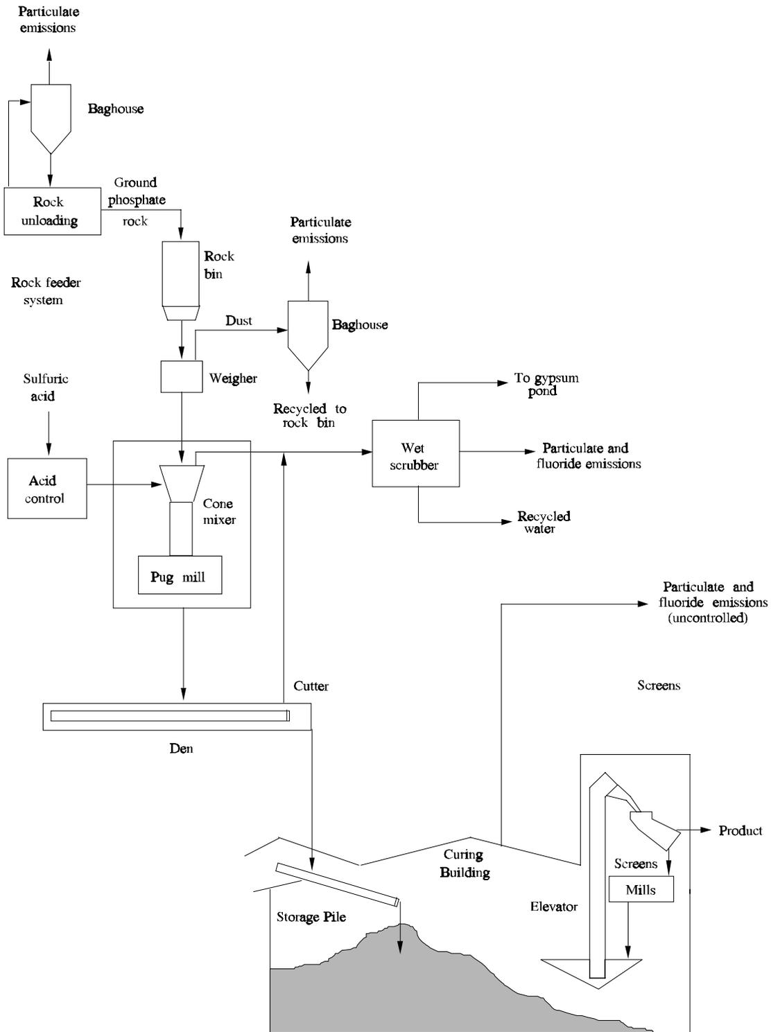
Figure 8.5.1-1. Normal superphosphate process flow diagram.<sup>1</sup>
