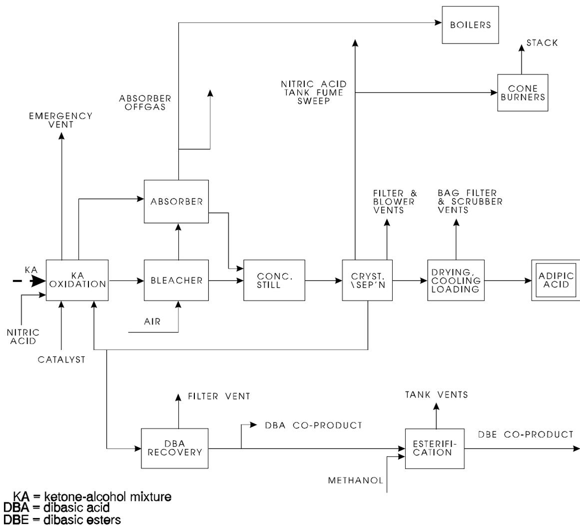
Figure 6.2-2. Adipic acid manufacturing process: Nitric acid oxidation of ketone-alcohol mixture.
