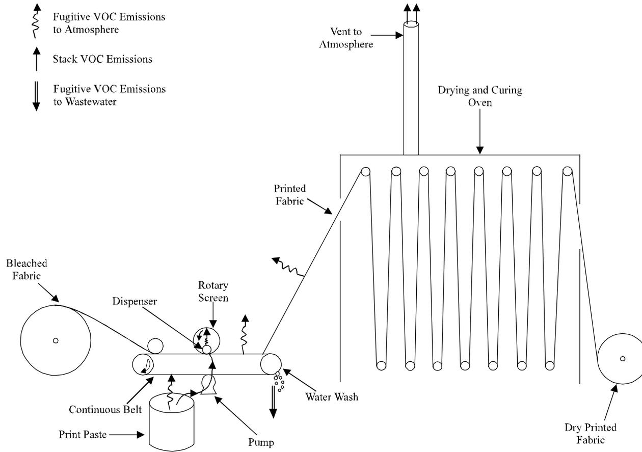
Figure 4.11-1. Schematic diagram of the rotary screen printing process, with fabric drying in a vented oven.
