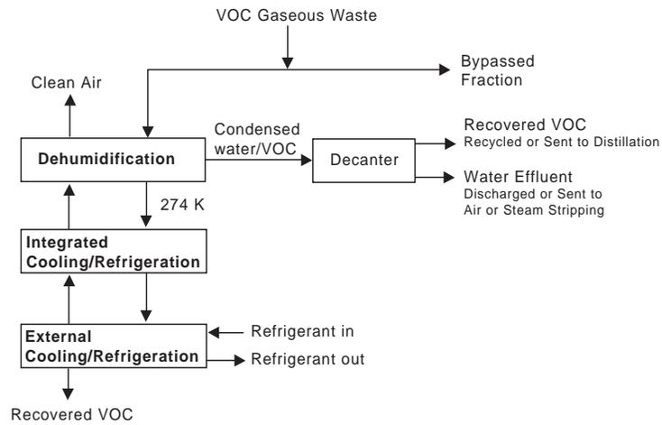
**Figure 2.2:** Schematic Diagram for a Refrigerated Condenser System
