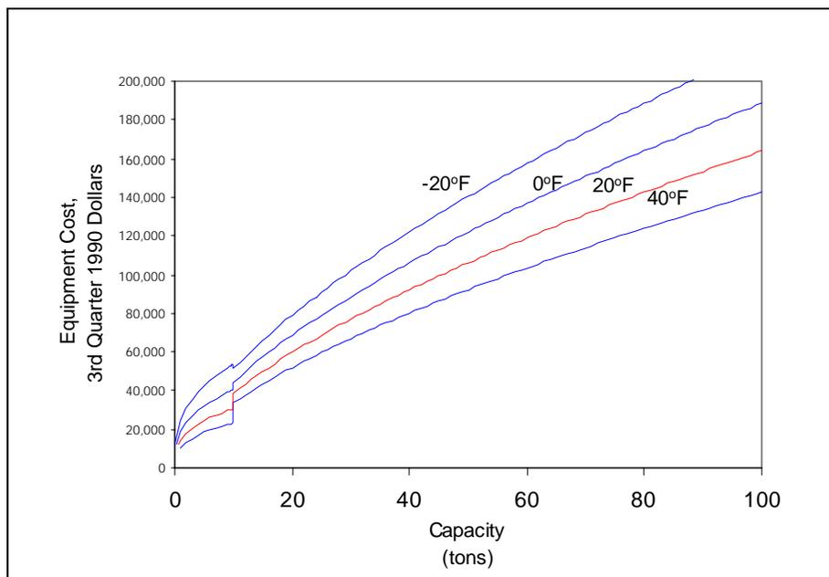
**Figure 2.5:** Refrigeration Unit Equipment Cost (Single Stage) [8.9]
