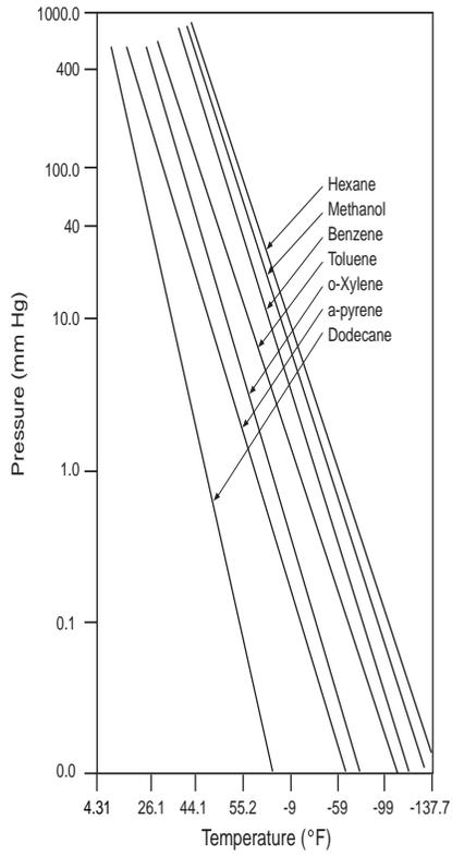
**Figure 2.1:** Vapor Pressures of Selected Compounds vs. Temperature [1]
