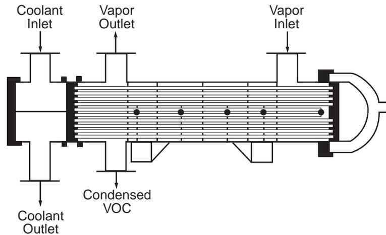
**Figure 2.3:** Schematic Diagram for a Refrigerated Condenser System
