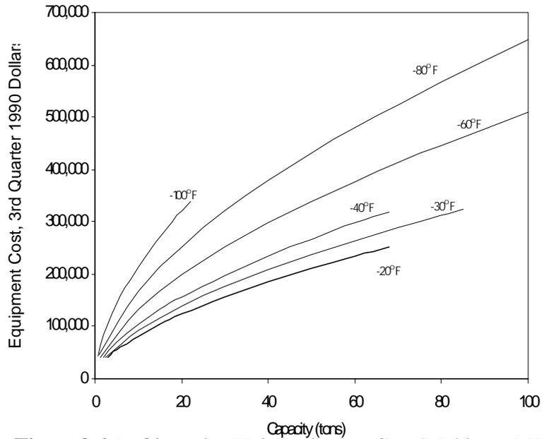
**Figure 2.6:** Refrigeration Unit Equipment Cost (Multistage) [9]
