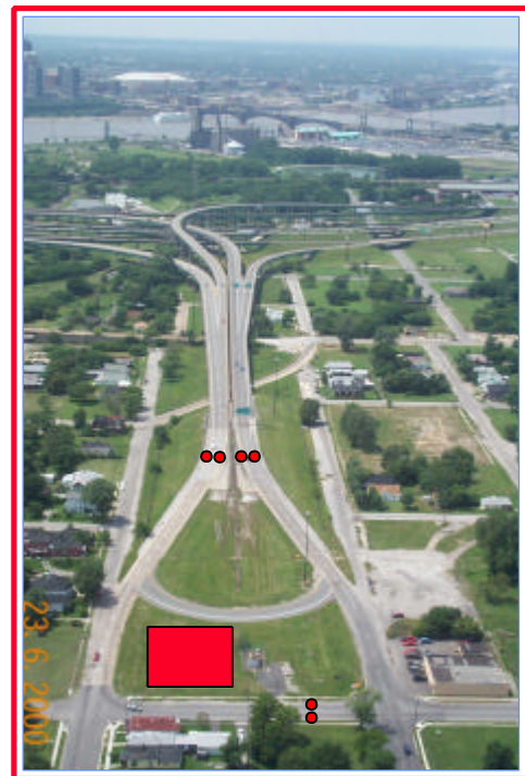
Figure 2. Approximate placement of the Numetrics "Groundhog" traffic sensors at the East St. Louis (IL) core site. Sensors denoted as red circles; Supersite monitoring footprint denoted as red rectangle.
