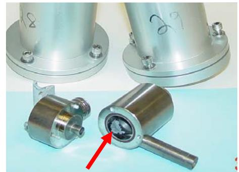
Speciation sampling canister with corrosion in cyclone.
