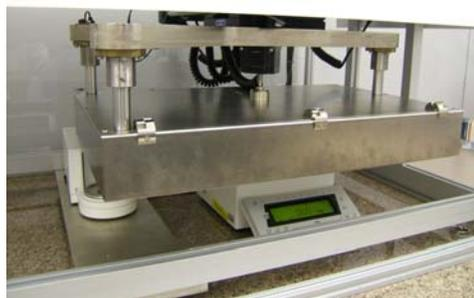
Filter tray enclosure during weighing
