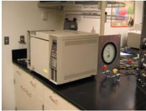
GC oven used to calibrate temperature devices
