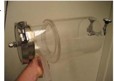
Isobaric chamber used to calibrate flow and pressure
