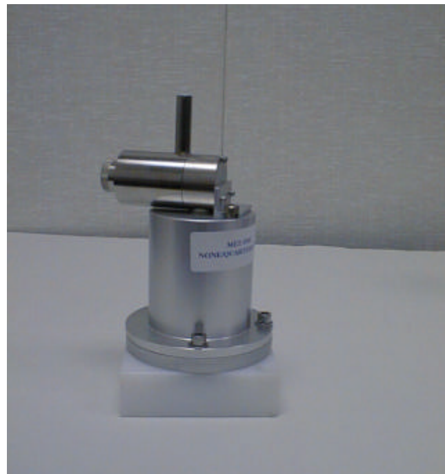
Sampling cassette with sharp cut cyclone (SCC)
