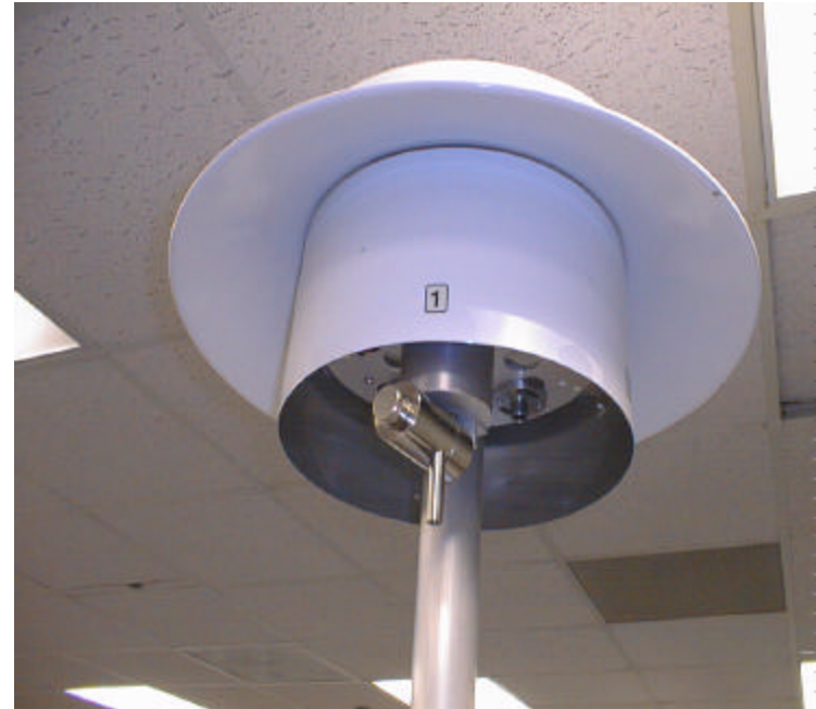
Solar shield with one sampling cassetted mounted
