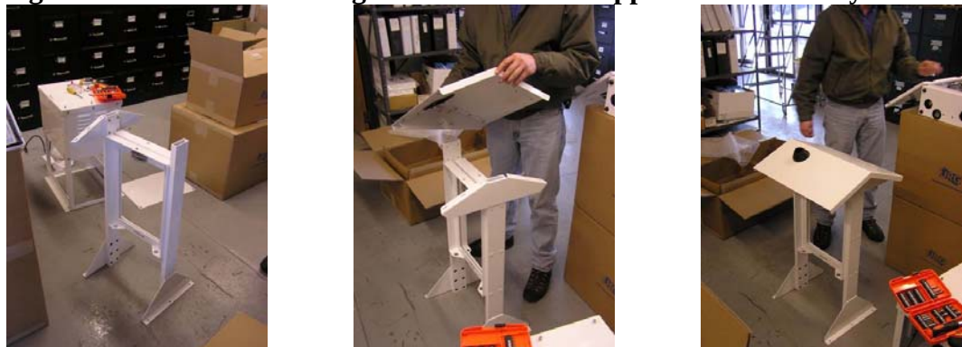
Figures C.7 to C.9. Installing the Second Roof Support to the H-Body
