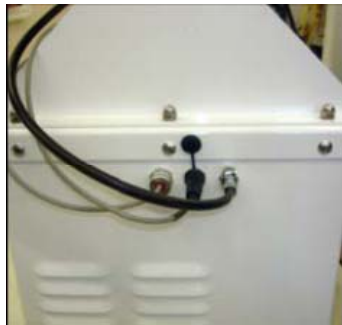
Figure 5.8 Vacuum (air) Line Disconnect
