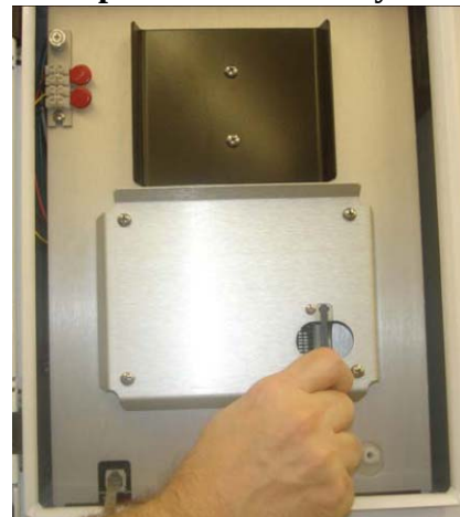
Figure C.28 Inserting the Compact Flash Memory Card
