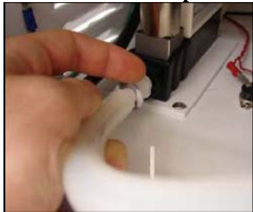
Figure 9.15 Disconnect Hose From MFC to Pump
