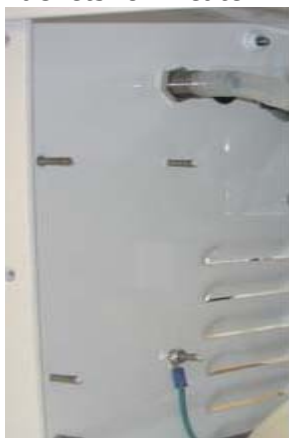
Figure 9.22 Four Mounting Brackets for Heater
