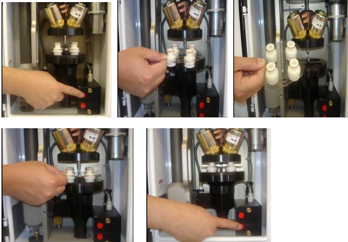
Figure 5.2 Replacement of Sample Cartridge with AUDIT Cartridge
