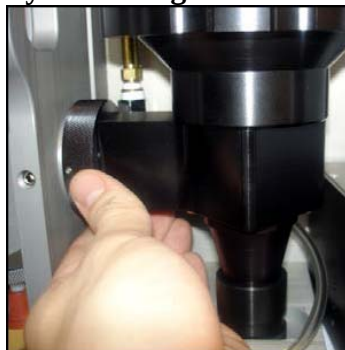
Figure 9.20 Unscrewing the Cyclone Ring
