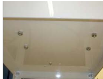
Figure 9.14 Remove Nuts from Bottom of Pump Enclosure
