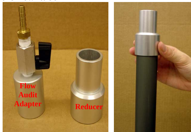
Figure 5.7 Placing the Reducer and the Flow Audit Adapter on the Downtube
