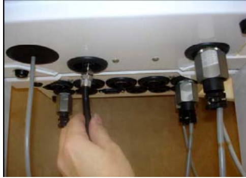
Figure C.23 Connection of Air Line to the Sample Module
