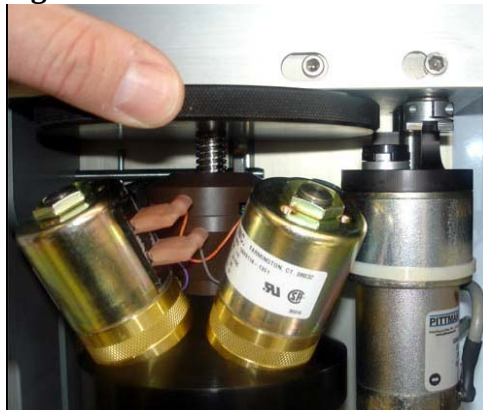
Figure 9.3 Use the Wheel to Raise and Lower Solenoid Manifold
