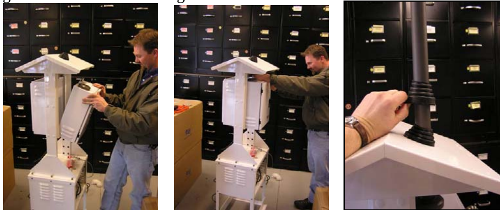
Figure C.15 to C.17 Inserting the Module Boxes and the Downtube
