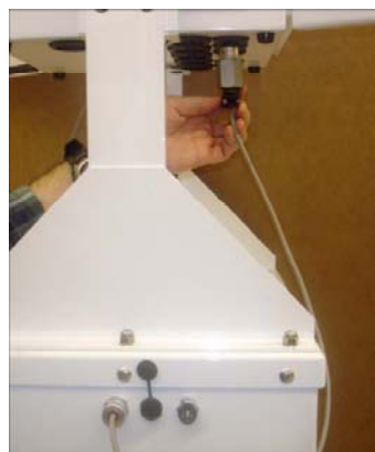
Figure C.18 Side View of Pump Relay Cable Connection
