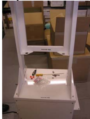
Figures C.10 to C.12 Installing of the Upright Support to the Base and the Proper Installation of the Support Feet
