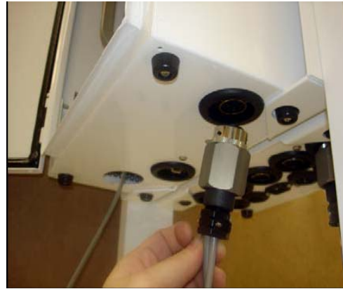
Figure C.22 Connection of the Controller Cable to Mass Flow Controller Connection on Lower Stand (Pump Enclosure)
