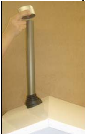
Figure 5.6 Removal of Ambient Air Inlet Cap
