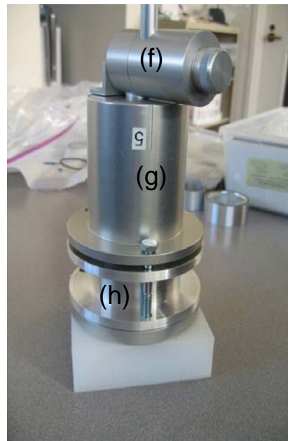
Figure 1b, SASS sampling mounted in plastic block for ease of handling. (f) sharp cut PM2.5 cyclone, (g) canister cover, (h) canister extender.
