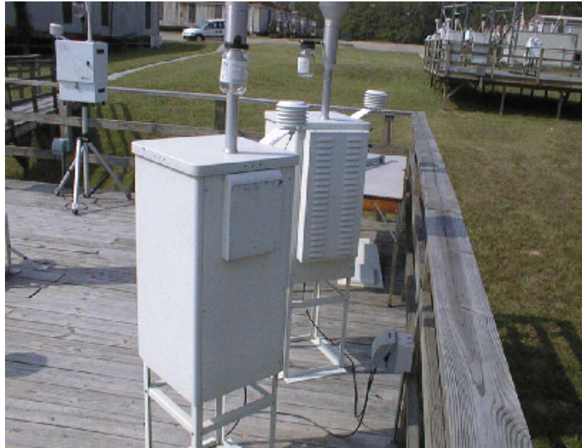
Figure 1. Showing the difference between the Andersen sequential's old back (on left) and the newer louvered back (on right) .
