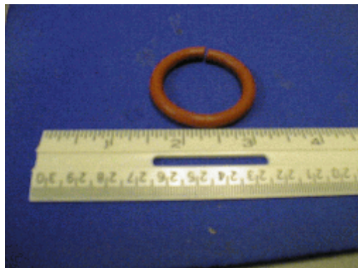
Figure 3. Showing a used red, rubber o-ring that was cut off of one of the main rotator wheels.
