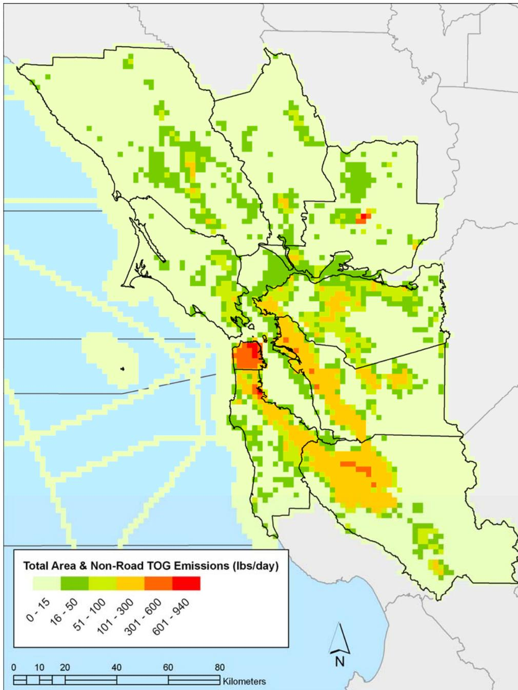
Figure 2-4. Emission density plot of area and non-road mobile source TOG emissions.
