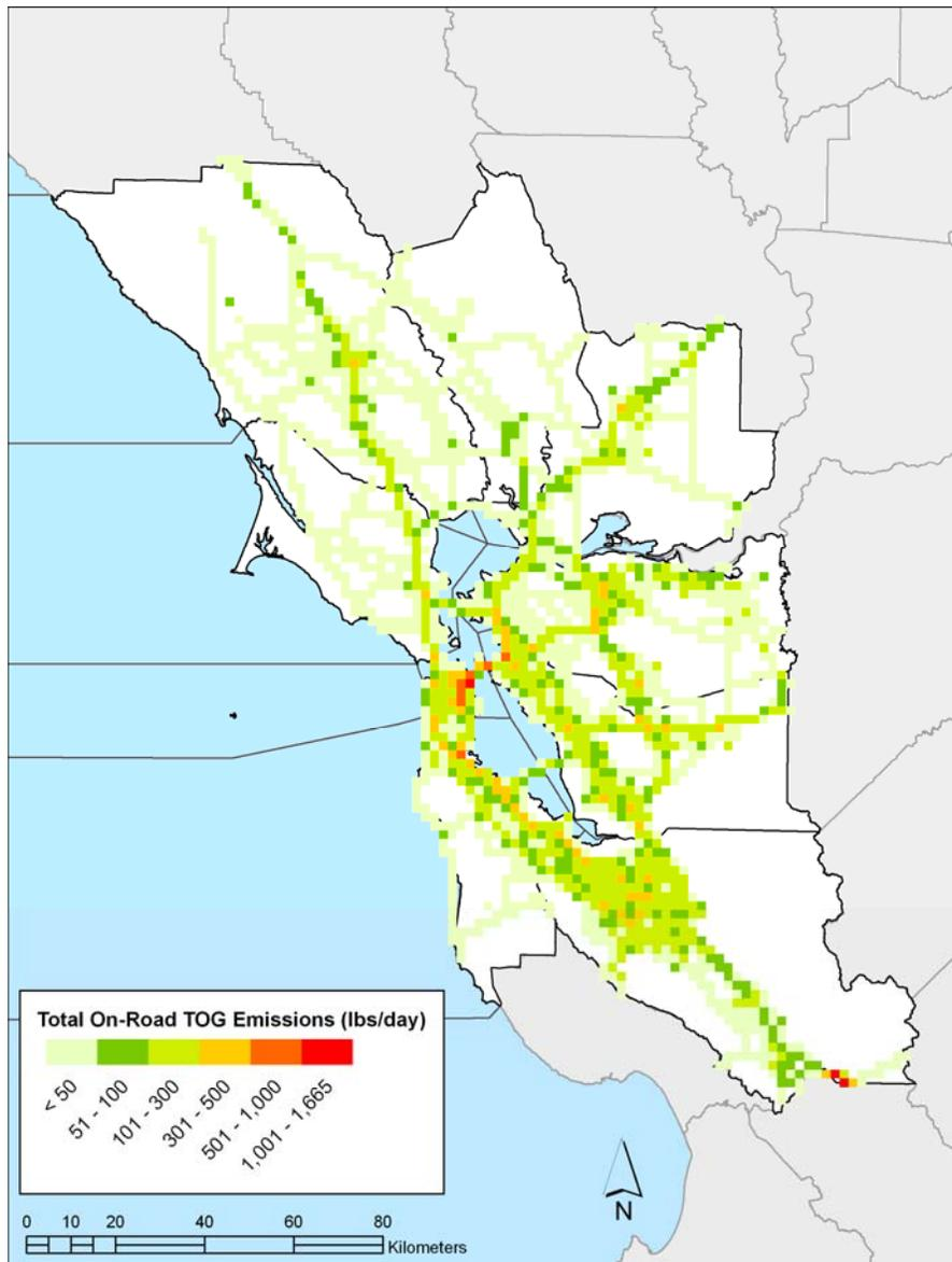
Figure 2-7. Emission density plot of on-road mobile source TOG emissions.
