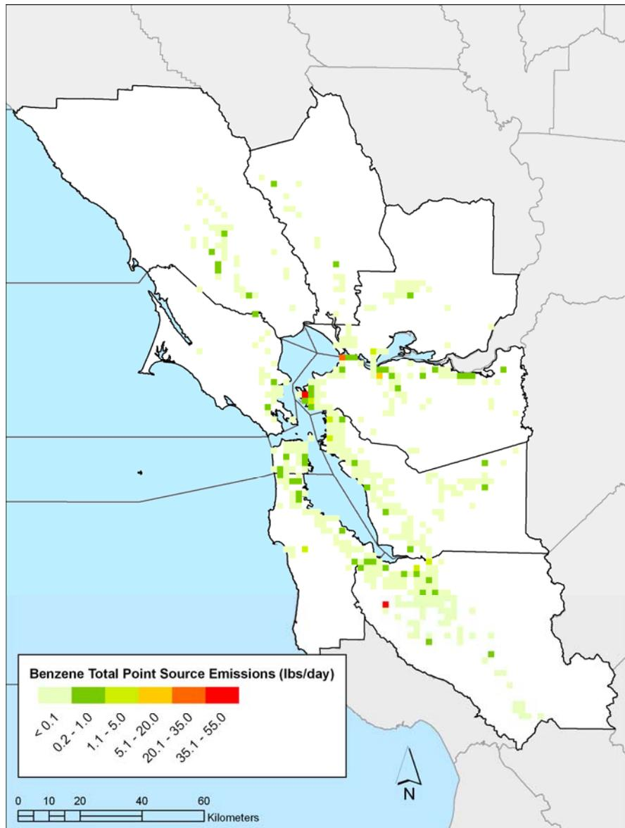
Figure 2-10. Emission density plot of benzene emissions from point sources.
