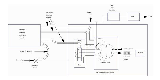
Figure 3. Automated Sampling and Analysis System for Cryogenic Trapping
