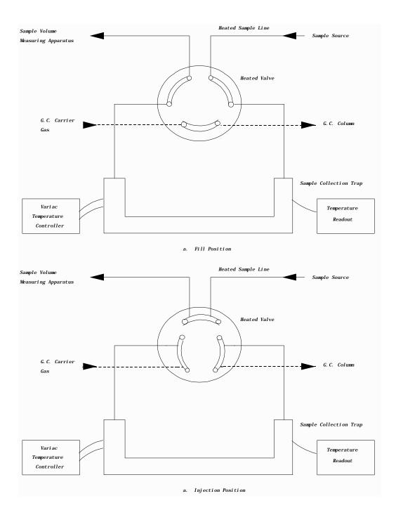
Figure 1. Schematic of Six-Port Valve Used for Sample Collection.
