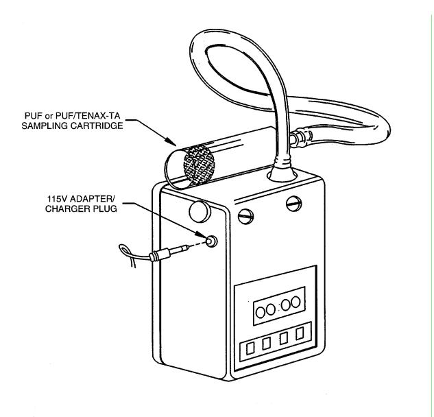
Figure 1. Low volume air sampler.
