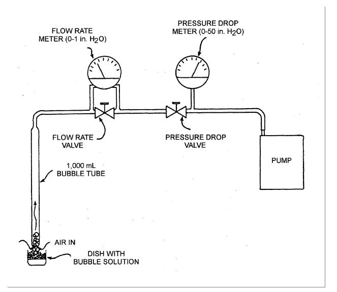
Figure 4. Calibration assembly for air sampler pump.
