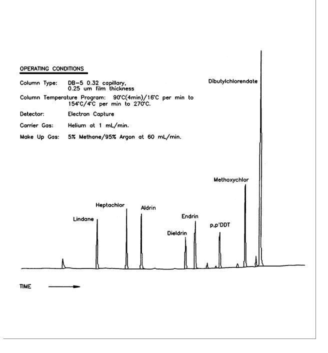
Figure 6. Chromatogram showing a mixture of single component pesticides determined by GC/ECD using a capillary column.
