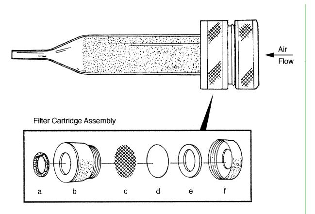
Figure 3. Open-face filter assembly attached to a PUF cartridge:(a) Inner Viton® o-ring, (b) filter cartridge, (c) stainless steel screen, (d) quartz filter, (e) filter ring, and (f) cartridge screw cap.
