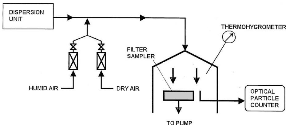
Fig. 1. Experimental set-up for the generation and collection of bioaerosols.
