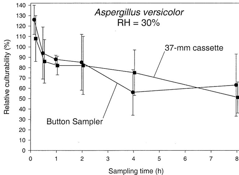
Fig. 3. Effect of sampling time on the relative culturability of *Aspergillus versicolor* spores at relative humidity (RH) of 30%. The error bars indicate the standard deviation of three repeats.
