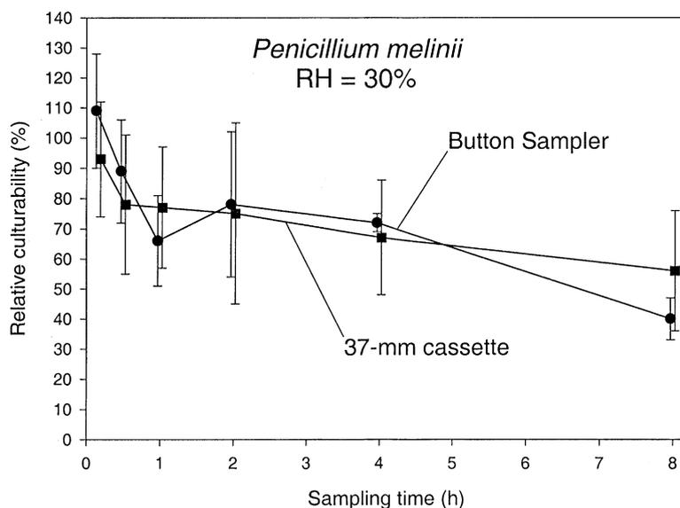
Fig. 2. Effect of sampling time on the relative culturability of *Penicillium melinii* spores at relative humidity (RH) of 30%. The error bars indicate the standard deviation of three repeats.
