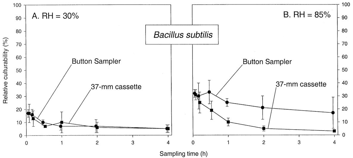
Fig. 4. Effect of sampling time on the relative culturability of *Bacillus subtilis* spores. The error bars indicate the standard deviation of three repeats. RH = relative humidity.
