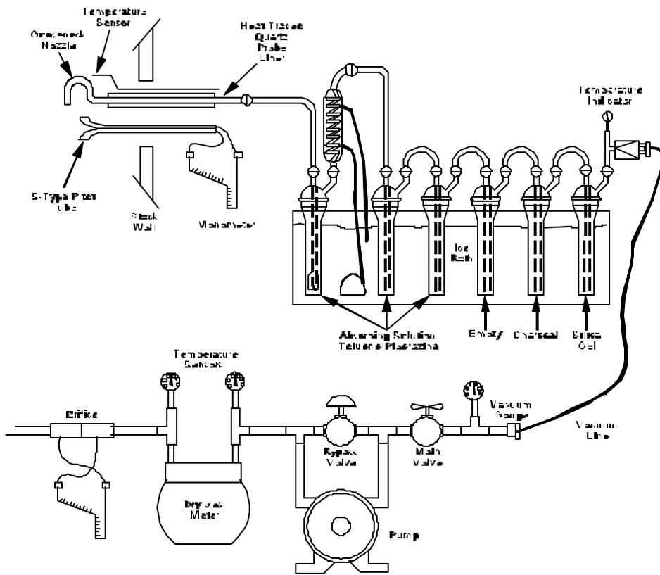
Figure 207-1-1. Sampling Train Configuration for Isocyanates
