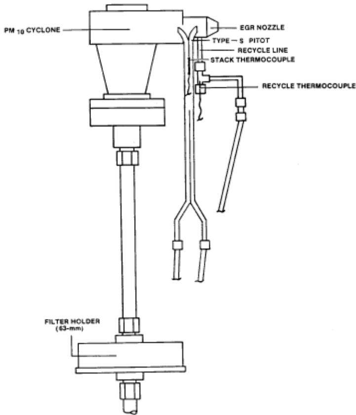
Figure 3. EGR PM<sub>10</sub> cyclone sampling device.
