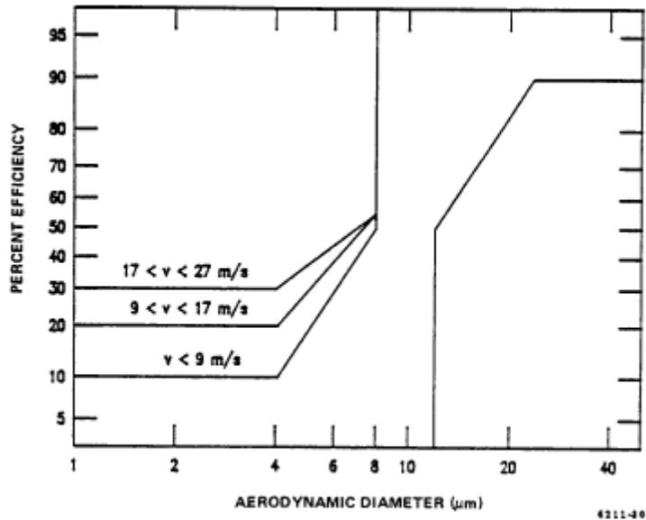
Figure 13. Efficiency envelope for the PM<sub>10</sub> cyclone.
