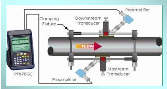
Section 2 has illustrations of state of the art instruments. This is an example of an ultrasonic flow meter.
