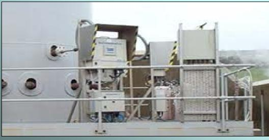
FTIR measurement system measuring stack gas concentrations in-situ
