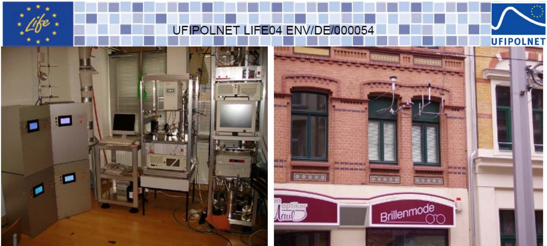
fig. 7.1a, b Photos of the 4 prototypes UFP 330 Sep-2006 at the common IfT/ UfZ (Helmholtz Zentrum für Umweltforschung – UfZ) calibration test laboratory in the Eisenbahnstr. in Leipzig situated in a flat. High polluted ambient air of a street canyon was measured. (Photo: TOPAS)
