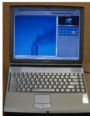
Commercial Computer Used to Processes Images With SCIENTECH Proprietary Software. Softgware Determines Opacity, Displays Results
