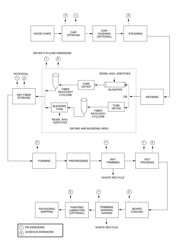
Figure 10.6.3-1. Typical process flow diagram for a medium density fiberboard (MDF) plant.
