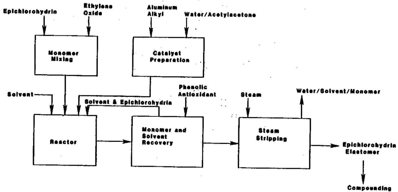
Figure 5. General flowsheet for the production of epichlorohydrin elastomers.<sup>1</sup>
