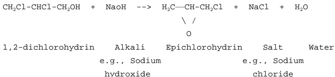
An excess of alkali drives the reaction to completion. The crude epichlorohydrin product stream (Stream 9) from the reactor contains 3 to 5 percent epichlorohydrin, other reaction products, and water.<sup>1,3</sup> The crude epichlorohydrin may be used directly in the production of glycerin or it may be refined for use in other manufacturing processes.
