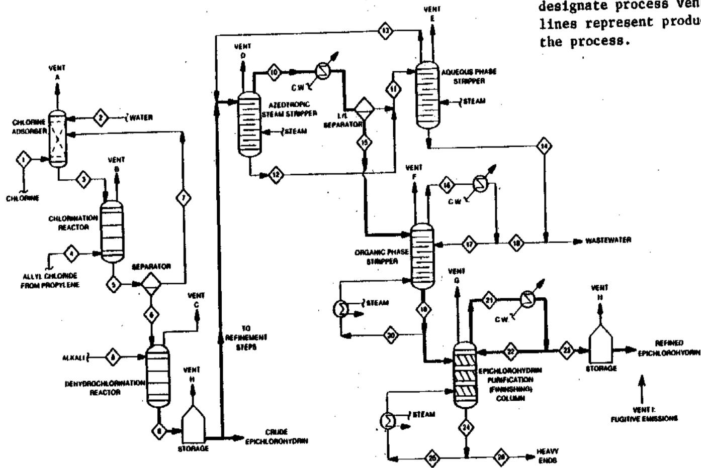
Note: The numbers in this figure refer to process streams, as discussed in the text. Letters designate process vents. Heavy lines represent product flow through the process.
