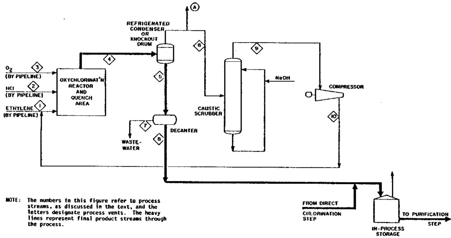
Figure 7. Basic operations that may be used in the production of ethylene dichloride by the balanced process, oxygen-based oxychlorination step.<sup>21</sup>
