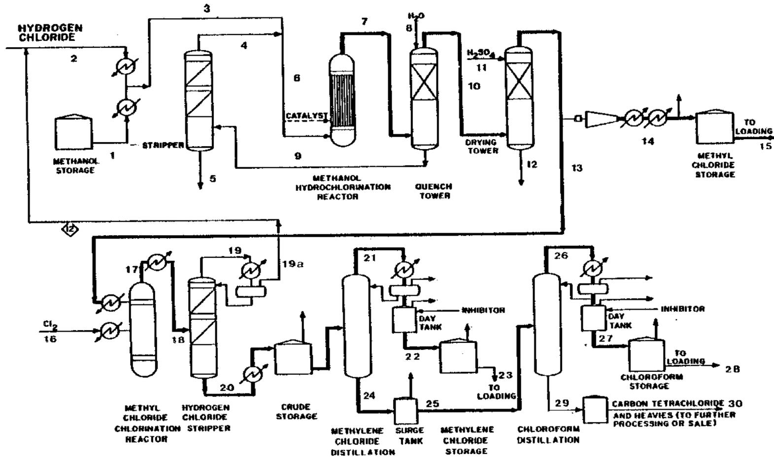
Figure A-1. Process flow diagram for hypothetical plant using methanol hydrochlorination, methyl chloride chlorination process showing stream numbers used in fugitive emission calculations.
