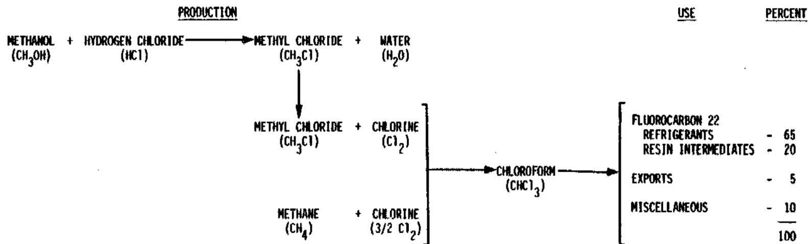
Figure 1. Chemical use tree for chloroform.<sup>7</sup>
