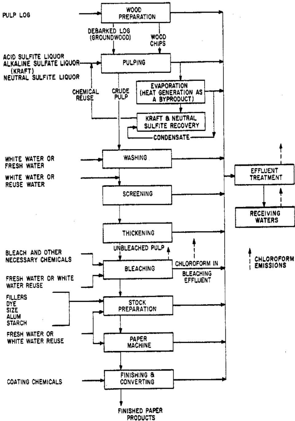
Figure 10. Basic operations that may be used in the pulp and paper manufacturing process.<sup>35</sup>
