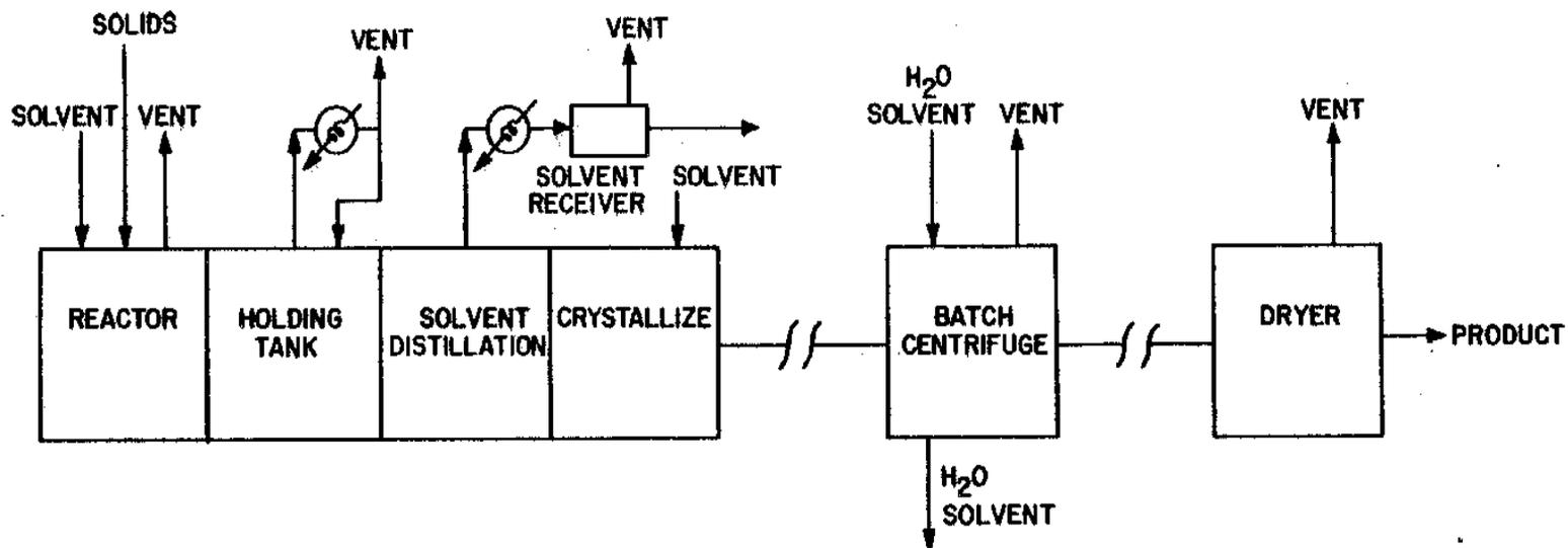
Figure 5. Basic operations that may be used in the synthetic pharmaceutical manufacturing process. 19
