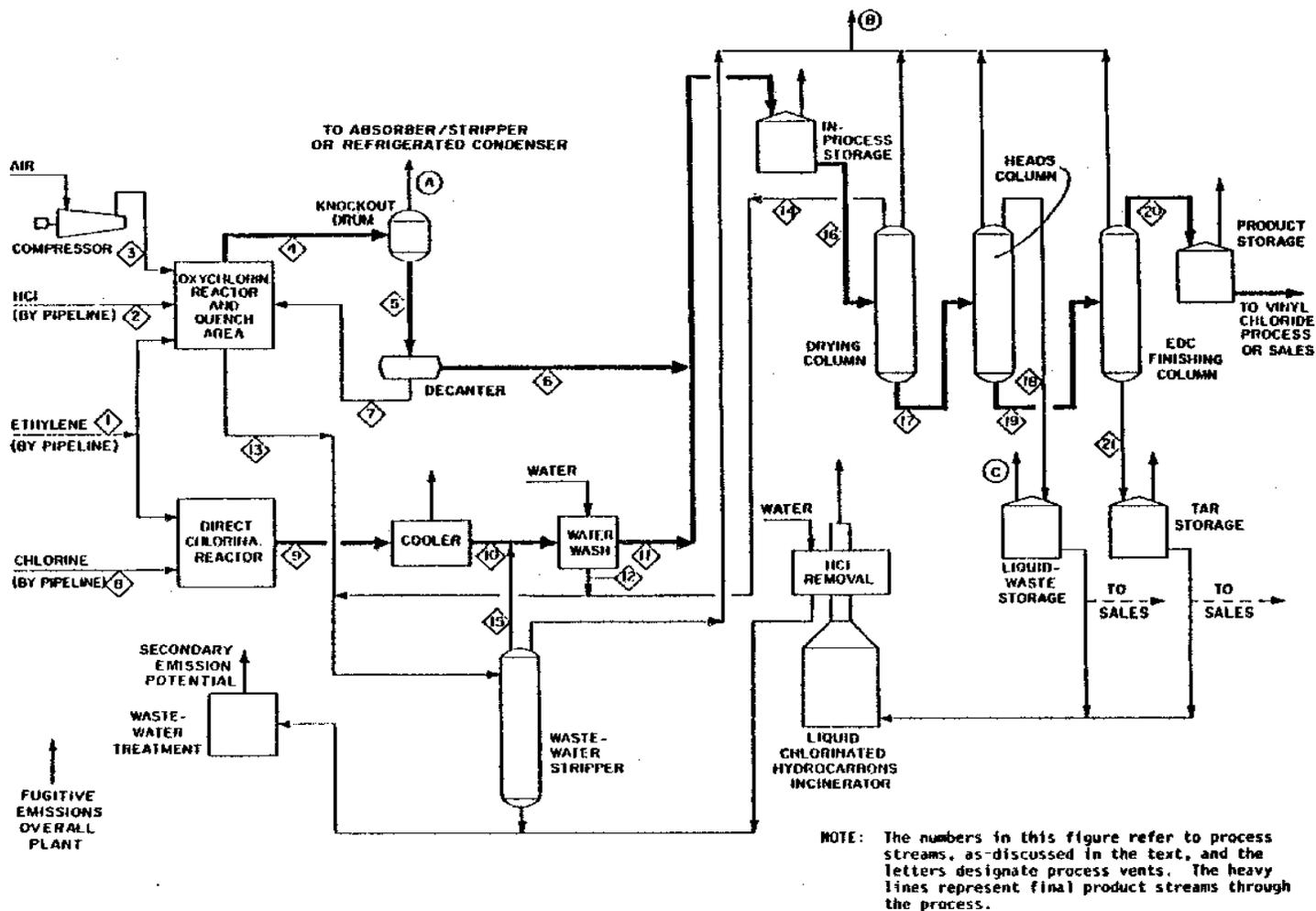
Figure 6. Basic operations that may be used in the production of ethylene dichloride by the balanced process, with air-based oxchlorination.<sup>21</sup>
