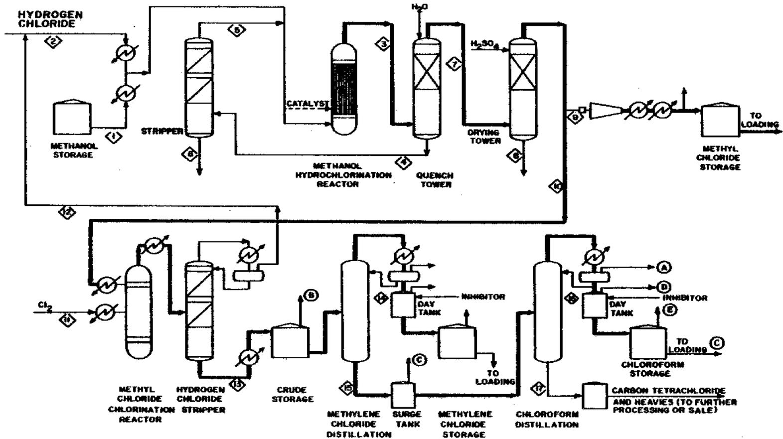
NOTE: The numbers in this figure refer to process streams, as discussed in the text, and the letters designate process vents. The heavy lines represent final product streams through the process.
