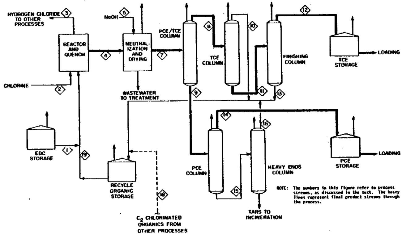
Figure 8. Basic operations that may be used in perchloroethylene and trichloroethylene production by chlorination of ethylene dichloride.<sup>33</sup>
