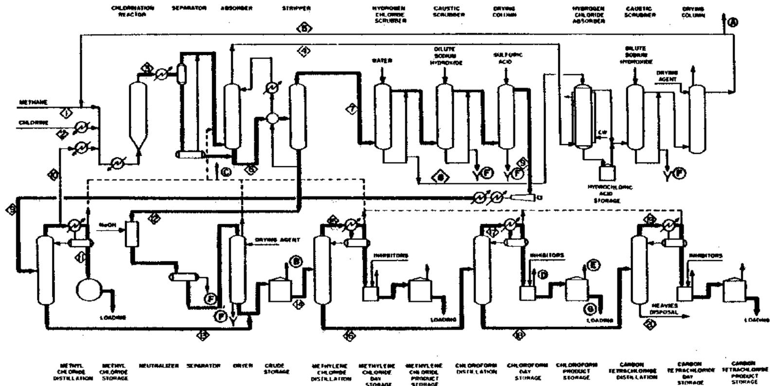
NOTE: The numbers in this figure refer to process streams, as discussed in the text, and the letters designate process vents. The heavy lines represent final product streams through the process.
