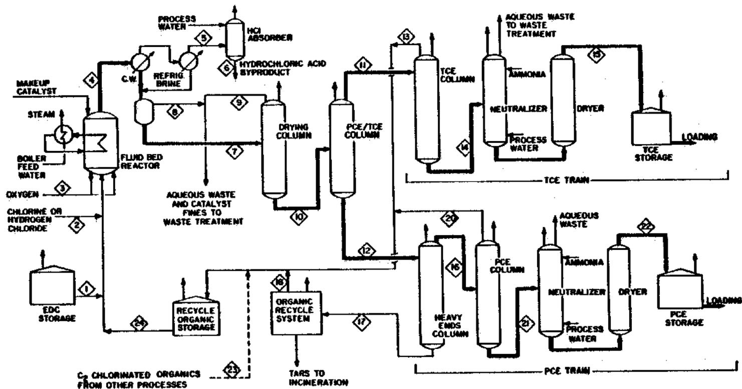
NOTE: The numbers in this figure refer to process streams, as discussed in the text. The heavy lines represent final product streams through the process.
