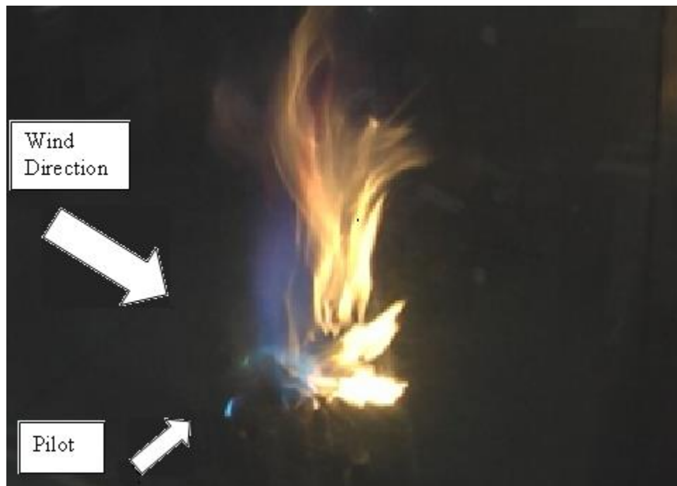
Figure 4 – Steam ring and pilots in operation with ethylene fuel (10kg/h ethylene and 20 kg/h steam).
