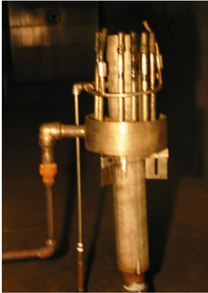
Figure 2 - Photo of steam ring with pilot burners
