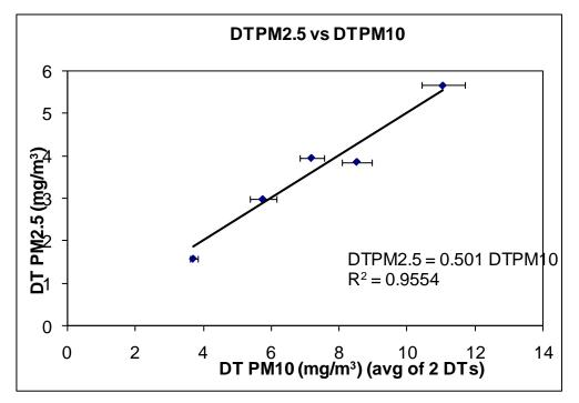
Figure 4-5. Comparison of Filter-Based PM<sub>2.5</sub> Mass Measurement With DustTrak Outfitted With PM<sub>2.5</sub> Inlet. Both instruments sampled silt material from the Phase IV tests that was resuspended in a specially designed chamber.
