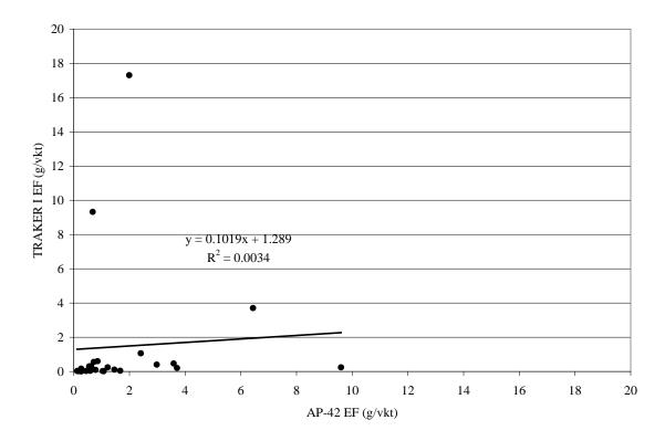
Figure 7-3. Scatter Plot of TRAKER I EF (g/vkt) versus AP-42 Silt-Based EF (g/vkt)
