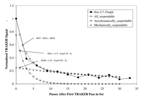
Figure 5-9. Normalized TRAKER I Decay Curve for Sets 4, 6, and 8 (45 mph measurement) and Hypothesized Aerodynamically Suspendable, Mechanically Suspendable, and Total Suspendable (aerodynamic plus mechanical) Road Dust Decay Curves
