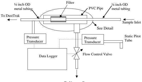
Figure 3-5. Isokinetic Inlet Schematic Diagram
