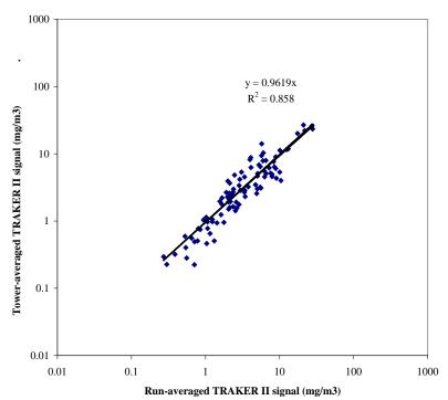
Figure 5-13. TRAKER II Ratio of Average of Left and Right Tire Inlet PM<sub>10</sub> Concentrations to Background (middle) Inlet PM<sub>10</sub> Concentration
