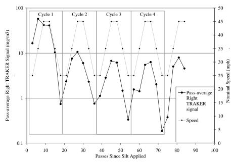
Figure 5-11. Speed Response of TRAKER I Signal. Figure shows the TRAKER I signal at each speed normalized to the average signal at 25 mph in the same cycle. Data are shown for 4 consecutive cycles as well as the average value for all cycles.
