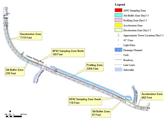
Note: The silt zone, with total length 2770 feet, includes Silt Buffer Zones, AP42 Sampling Zones, and Profiling Zone.
