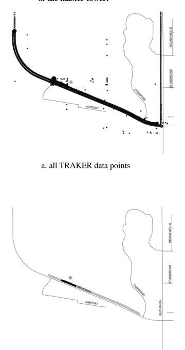
b. Data filtered for validity and location on test route and/or within 50 m of master tower.
