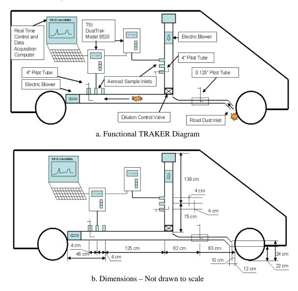
Figure 3-10. Schematics and Dimensions of TRAKER II
