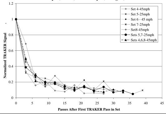
Figure 5-8. Normalized TRAKER I Decay Curve for Sets 5 and 7 (25 mph measurement) and Hypothesized Aerodynamically Suspendable, Mechanically Suspendable, and Total Suspendable (aerodynamic plus mechanical) Road Dust Decay Curves
