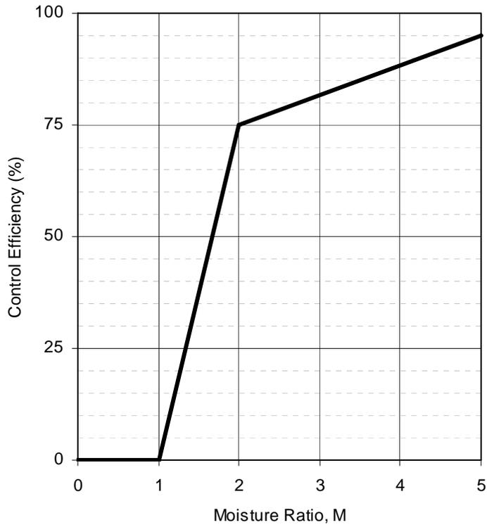
Figure 13.2.2-2. Watering control effectiveness for unpaved travel surfaces
