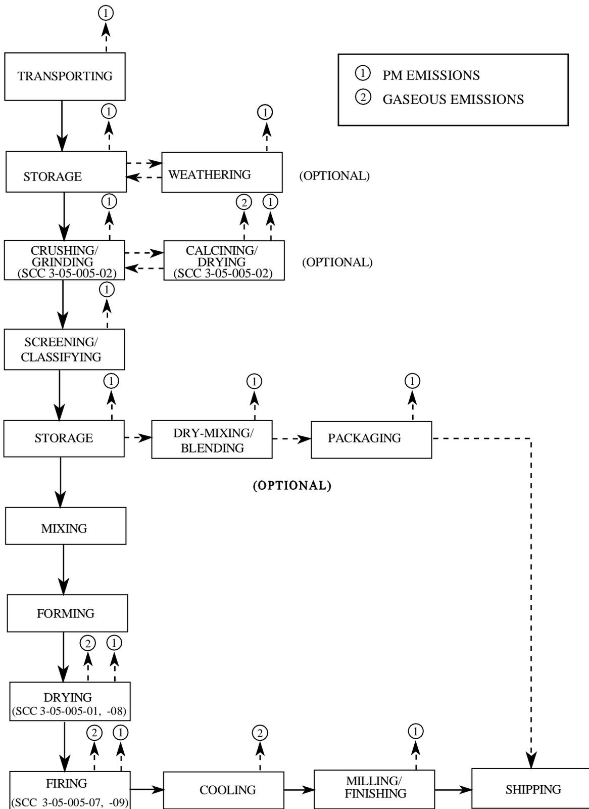
Figure 11.5-1. Refractory manufacturing process flow diagram.<sup>1</sup>
