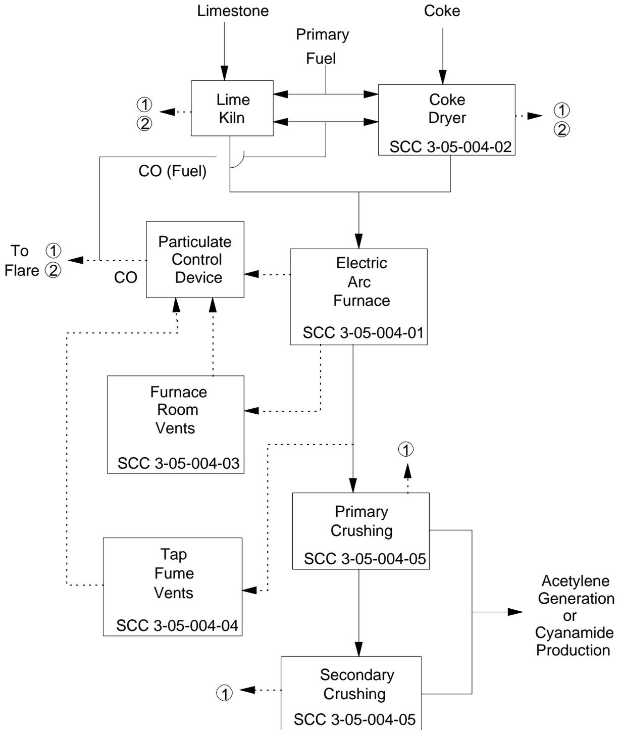
Figure 1. Process flow diagram for calcium carbide manufacturing (SCC = Source Classification Code).
