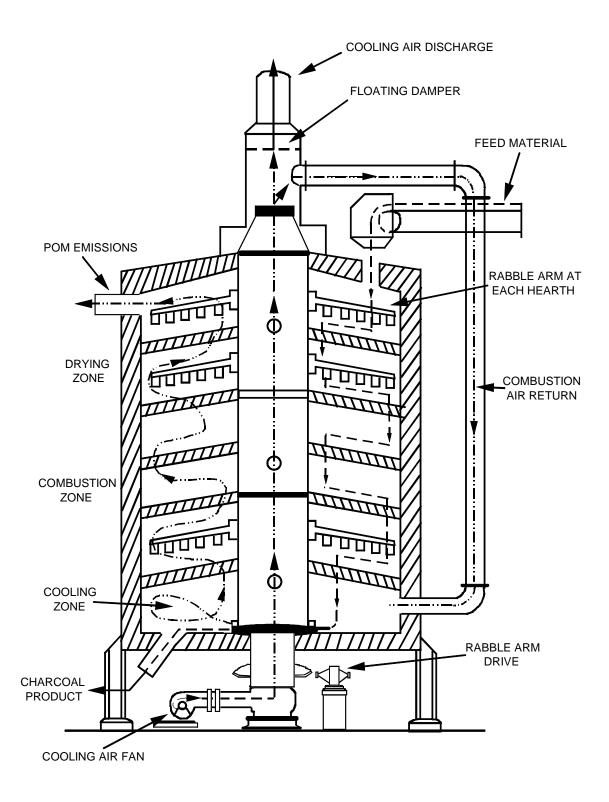
Figure 10.7-2. The continuous multiple hearth kiln for charcoal production.<sup>4</sup> (Source Classification Code: 3-01-006-04.)
