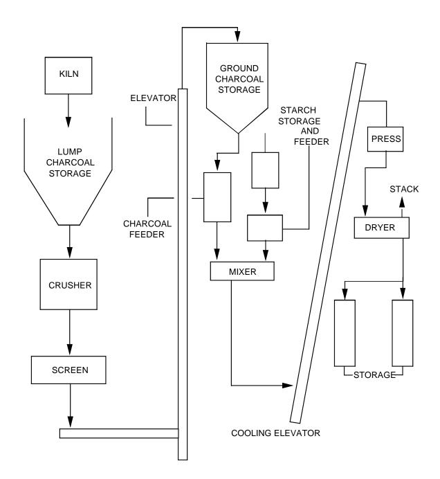
Figure 10.7-3. Flow diagram for charcoal briquette production.<sup>3</sup> (Source Classification Code: 3-01-006-05.)
