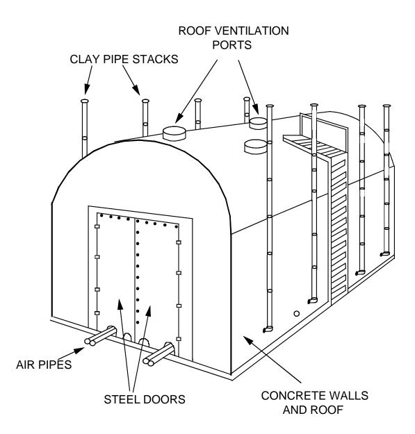
Figure 10.7-1. The Missouri-type charcoal kiln.<sup>7</sup> (Source Classification Code: 3-01-006-03.)
