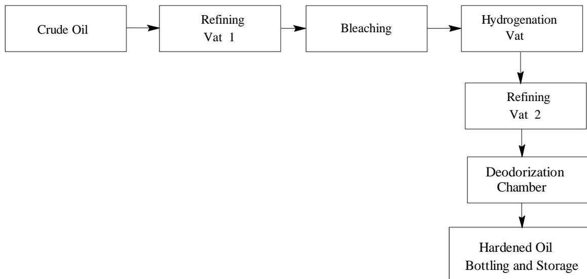
Figure 9.13.1-4. Oil hardening process.
