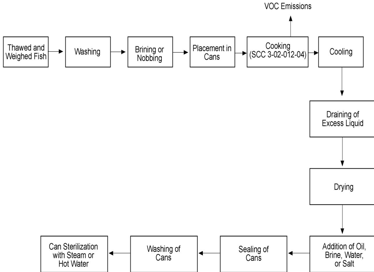
Figure 9.13.1-2. Flow diagram of raw packing method.
