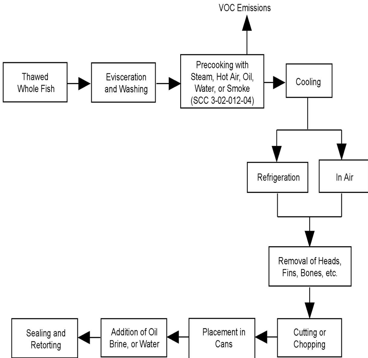
Figure 9.13.1-1. Flow diagram of precooking method.
