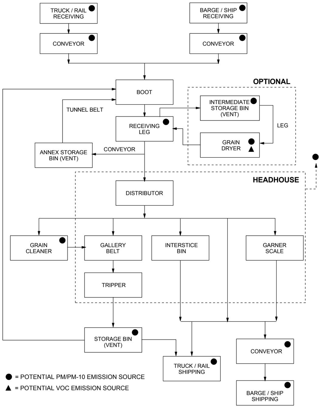
Figure 9.9.1-1. Major process operations at a grain elevator.
