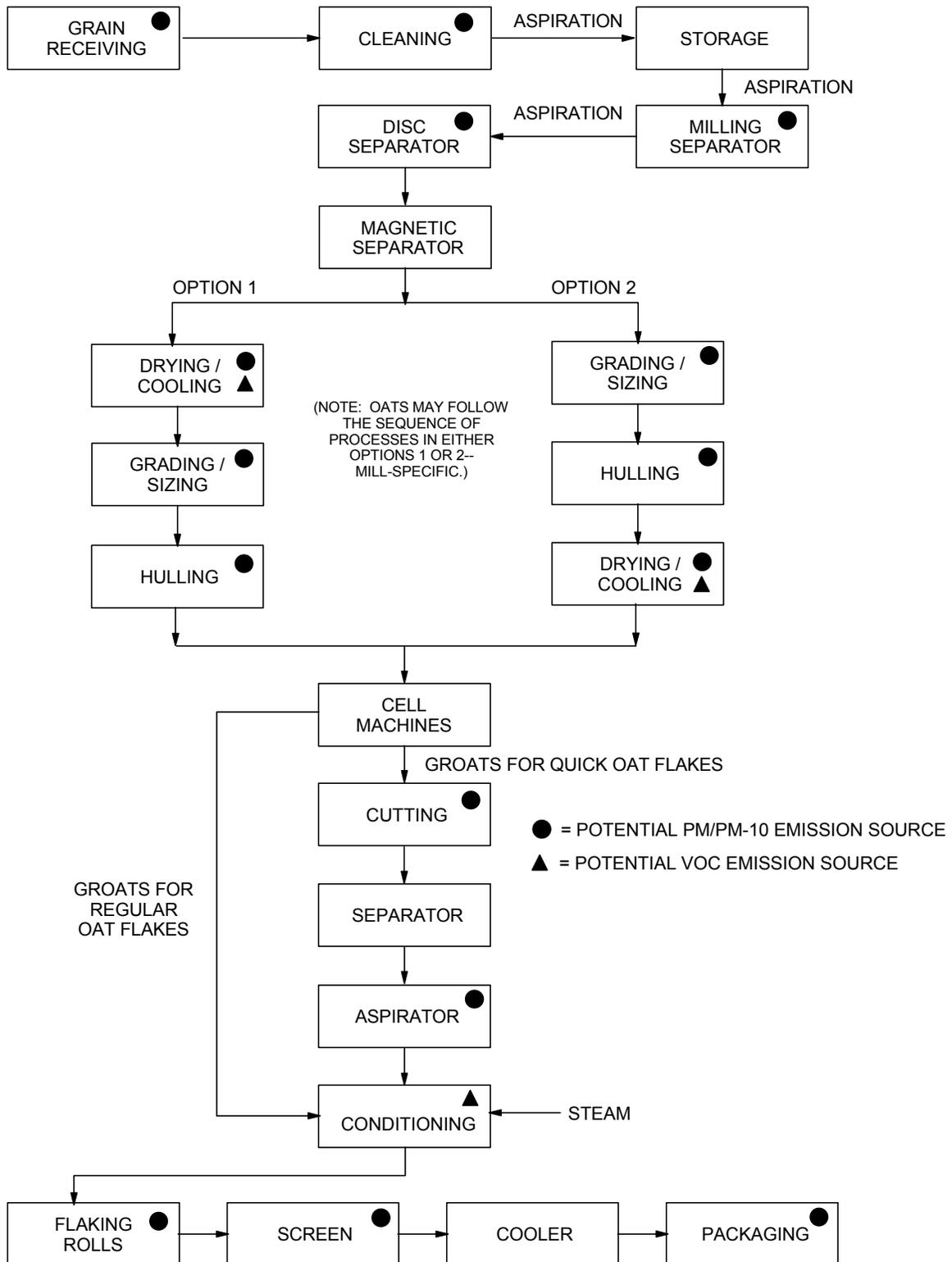
Figure 9.9.1-3. Flow diagram for oat processing operations.<sup>8</sup>
