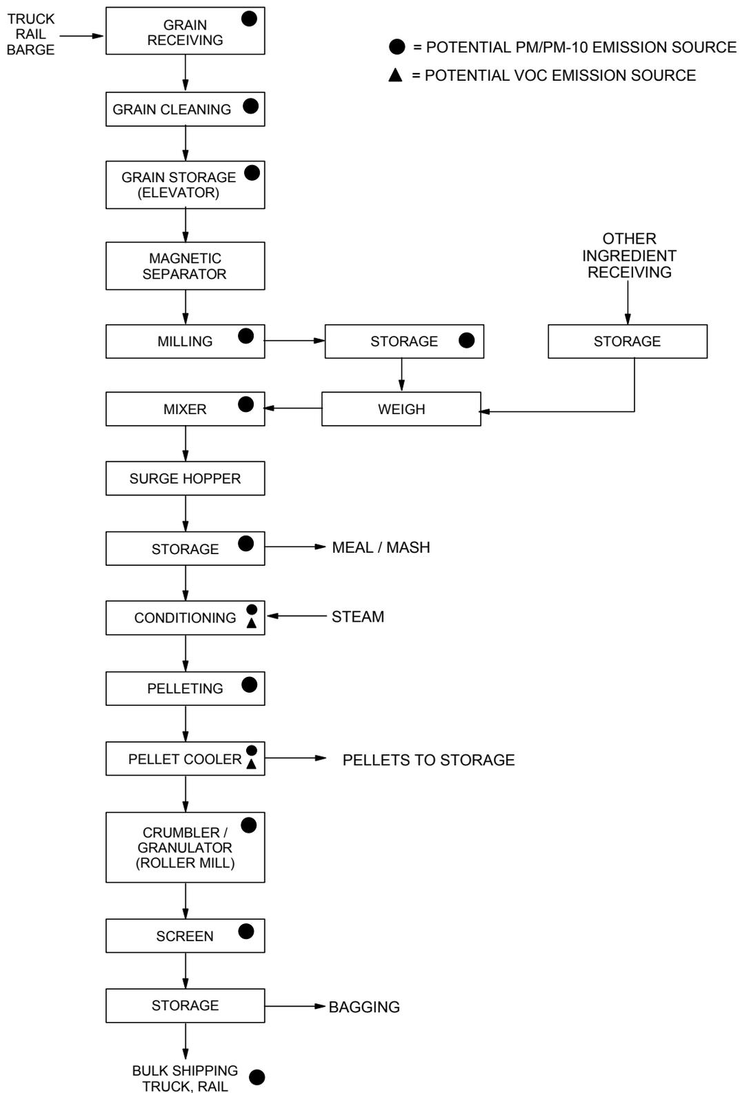
Figure 9.9.1-6. Typical animal feed milling process flow diagram.
