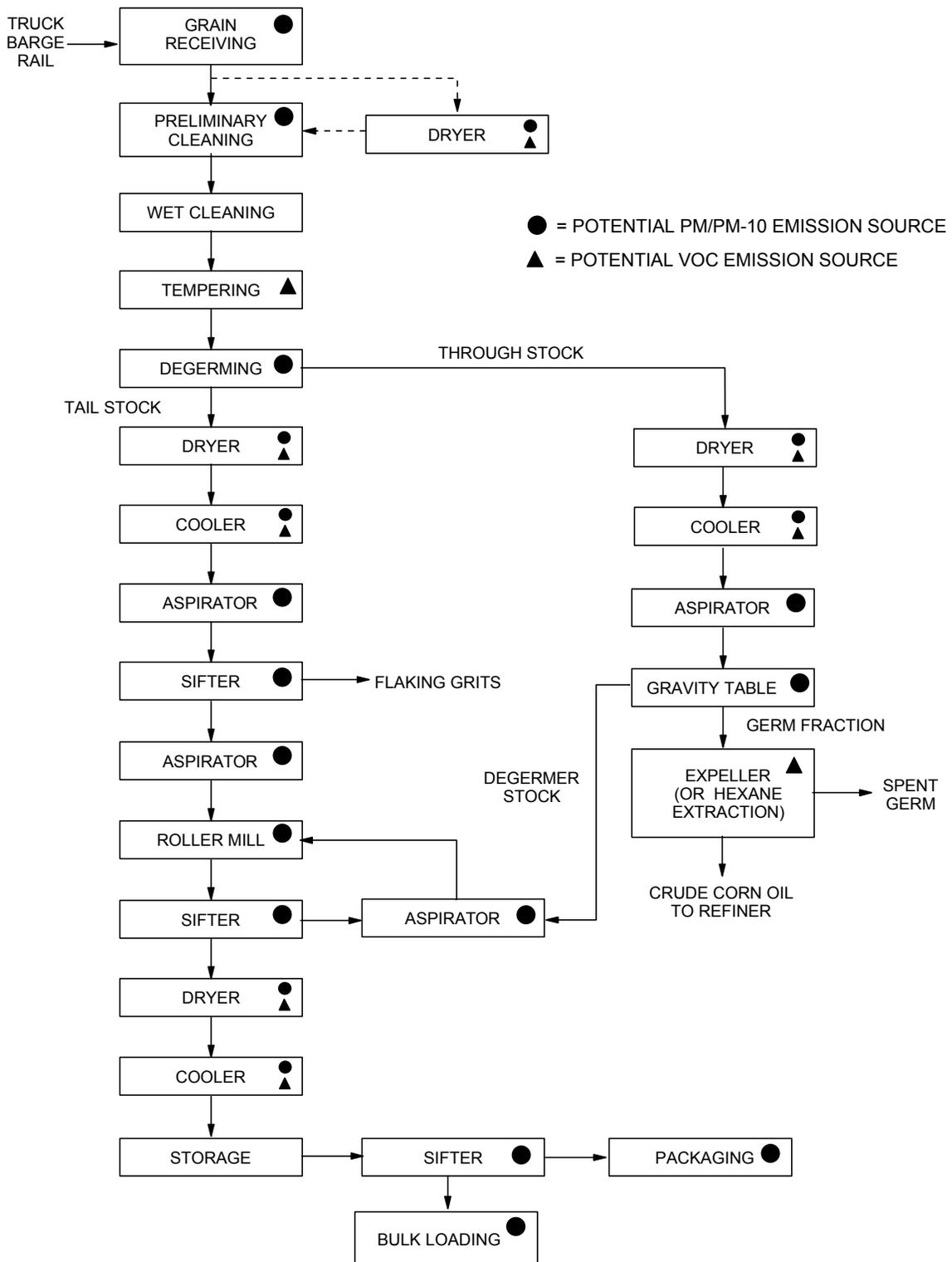
Figure 9.9.1-5. Simplified process flow diagram for a corn dry milling operation with degerming.
