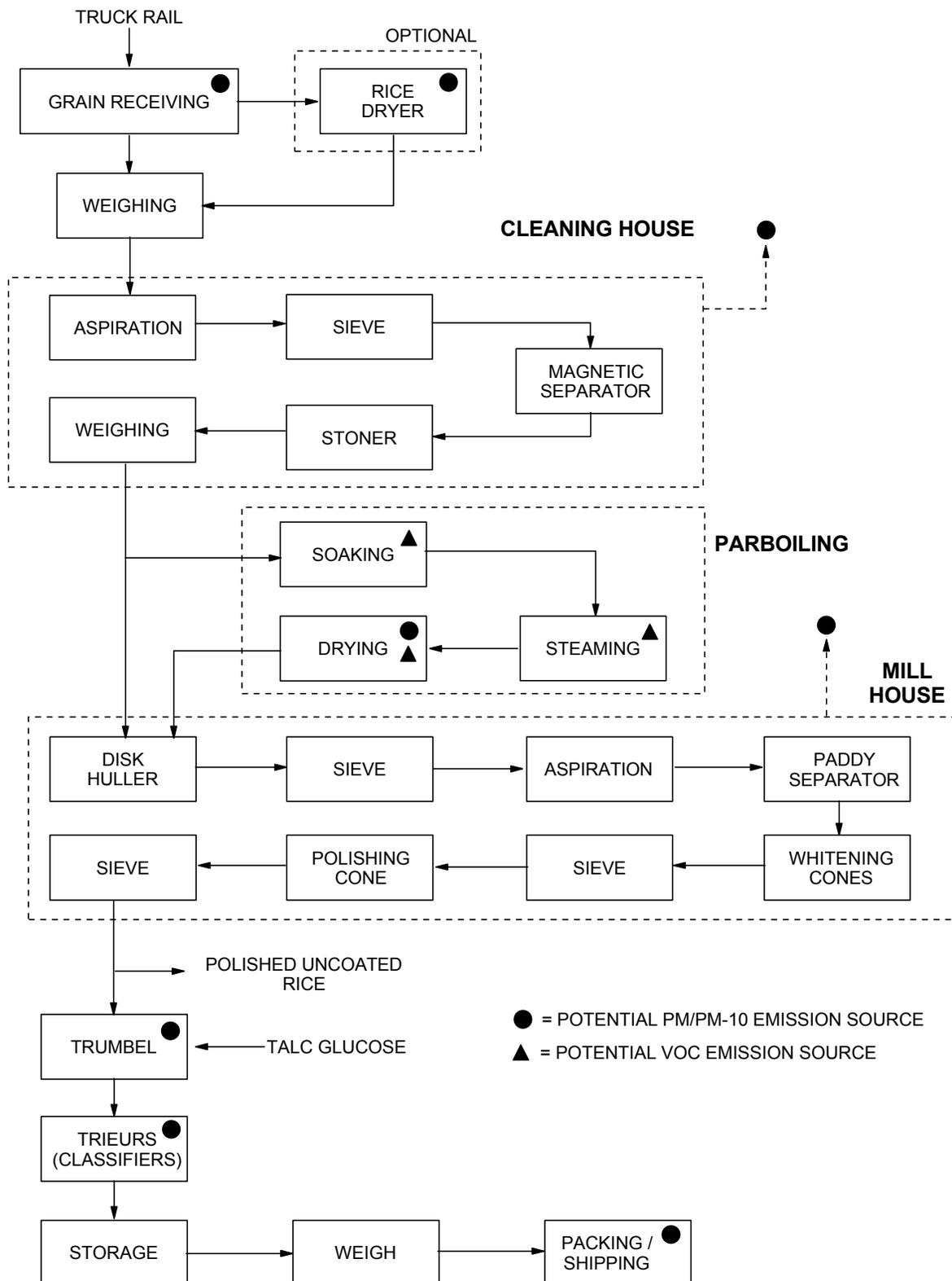
Figure 9.9.1-4. Flow diagram for conventional and parboil rice mills.
