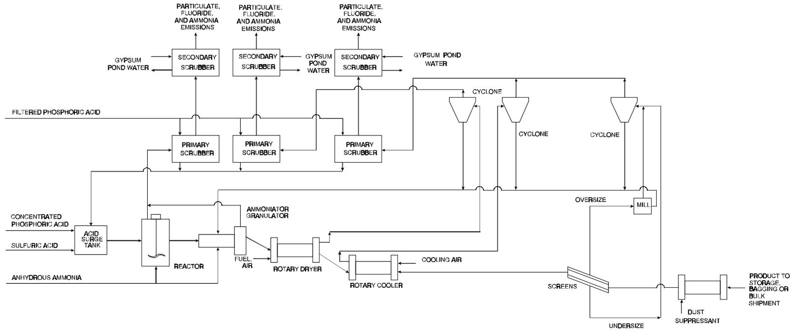
Figure 8.5.3-1. Ammonium phosphate process flow diagram.
