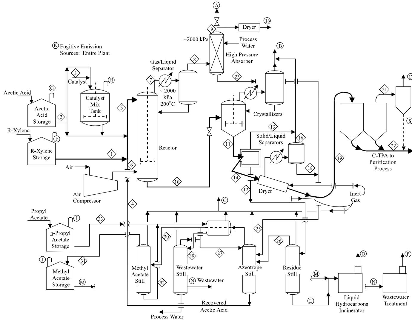
Figure 6.11-1. Crude terephthalic acid process.
