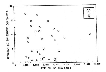
Figure 4-1. Unweighted  $\mathrm{NO}_{\mathrm{X}}$  and CO emissions versus engine ratings for diesel engines greater than 600 hp.
